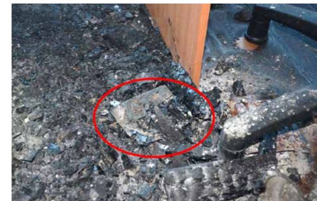
The PCB (circuit board) lying amongst debris on the floor
