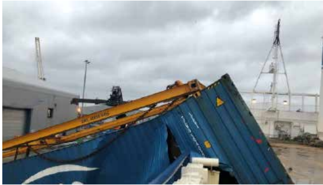
A container has been ripped open following wires breaking; the cargo inside was damaged
