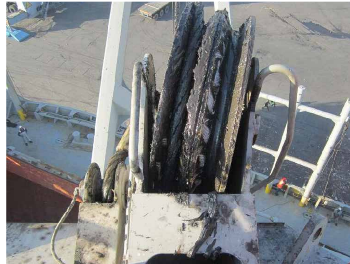
This image shows a wire sheave which has been damaged
