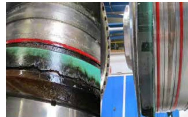
'Dieseling effect' visible on hydraulic cylinders
