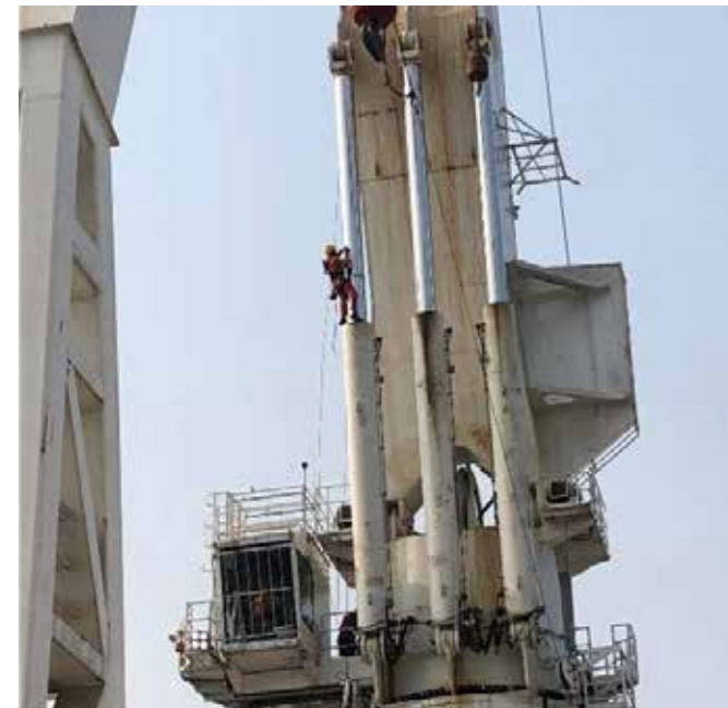
Damage to hydraulic cylinders due to contact with containers while loading / unloading
