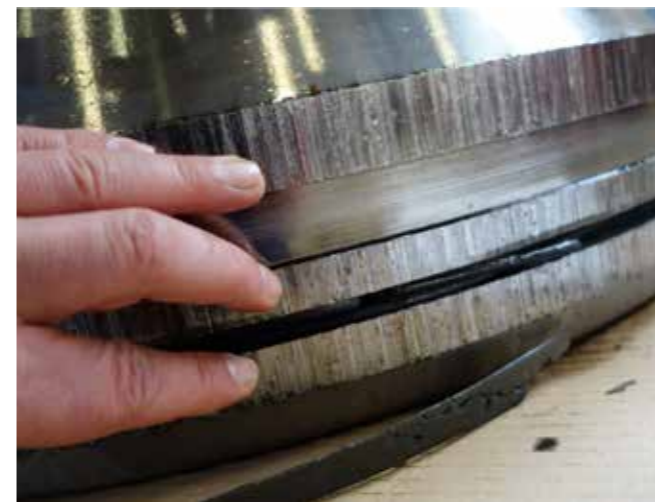
Abrasive damage to the CPP hub piston
