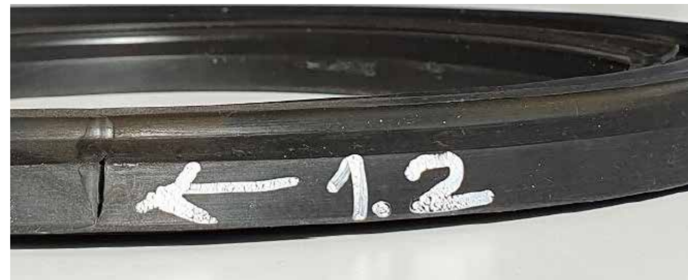
Propeller blade seals - poor ring joint bonding/seal twisted
