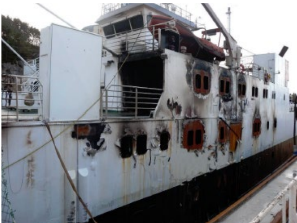
An example of fire damage seen by Norwegian Hull Club that resulted from Hot Work
