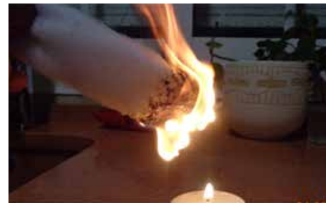
The polyester filter material is extremely flammable
