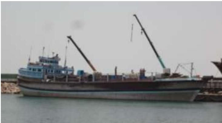
*Key Identification features:* It has a characteristic keel design, with a sharp curve right below the top of the prow. The Sambuq can have rounded or squared stern.
