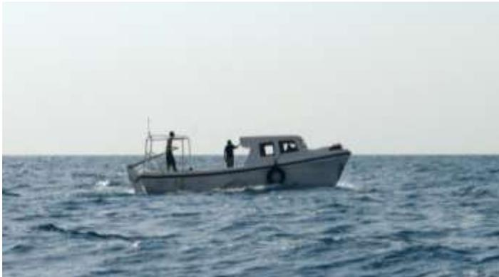
Skiff with Semi displacement hull and a small cabin in front.
